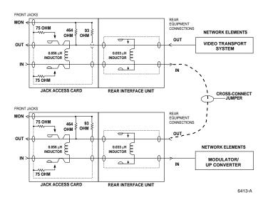
Figure 17. Typical Cross-Connect Application
